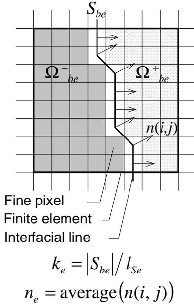
Fig. 5. Definition of geometric parameters in element
