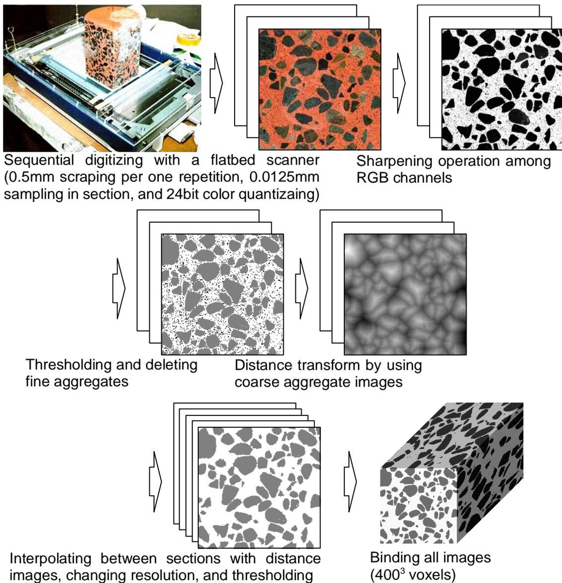
Fig. 1. Image digitizing and processing procedure
