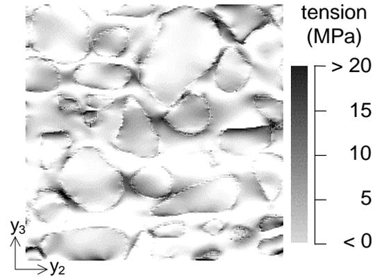
Fig. 3. Maximum principal stress in the center of  $y_2$ - $y_3$  section
