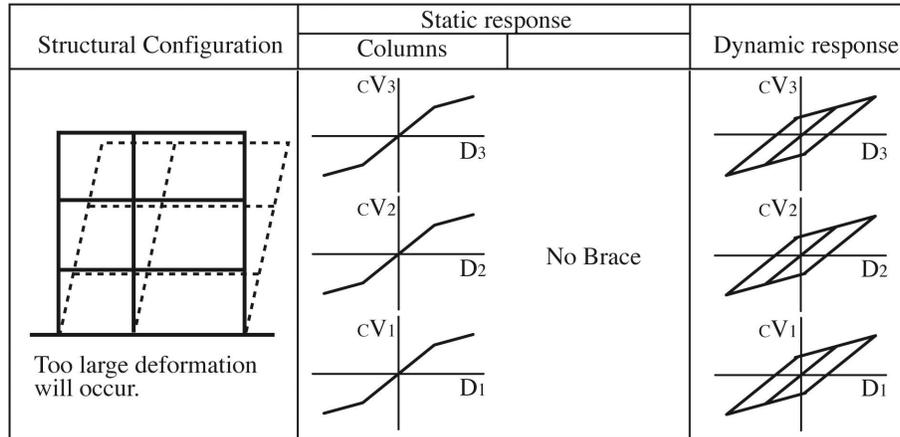
Fig. 3-a Earthquake Response of Moment Resisting Frame
