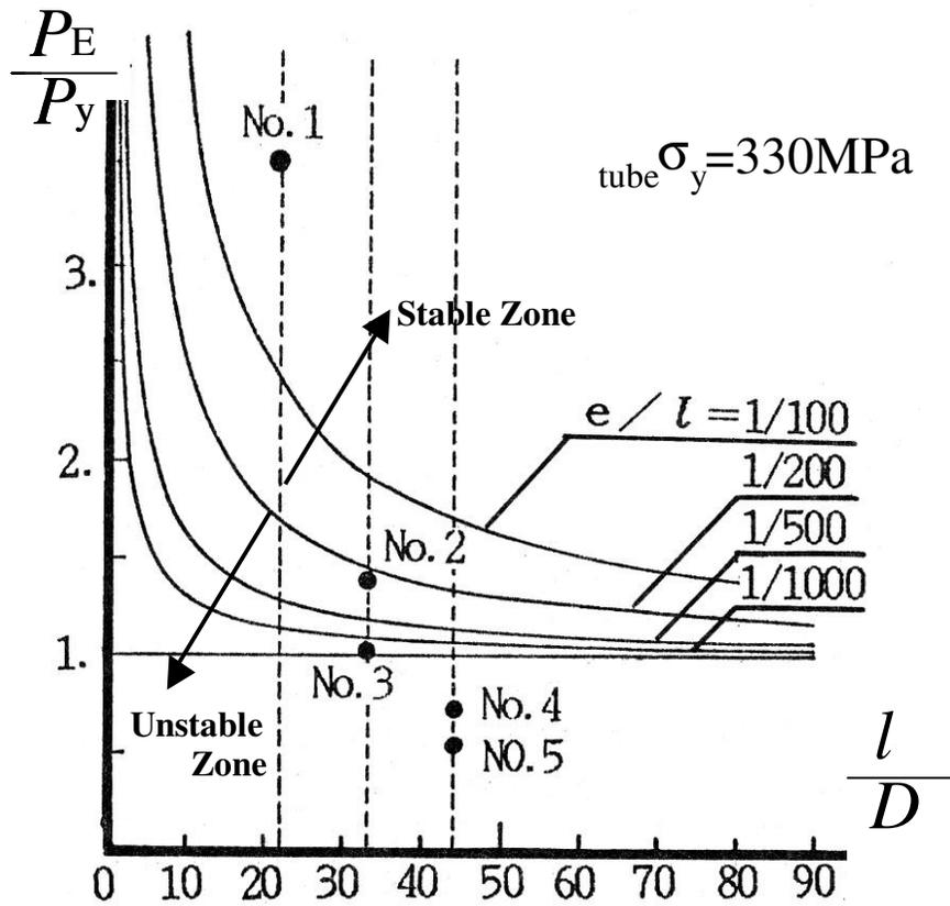
Fig. 14 Stability Chart for Buckling Restrained Braces
