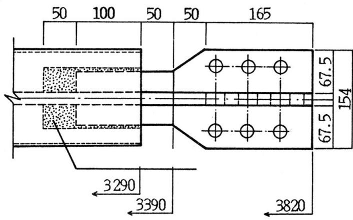
Fig. 6 Right End Detail of the Specimen
