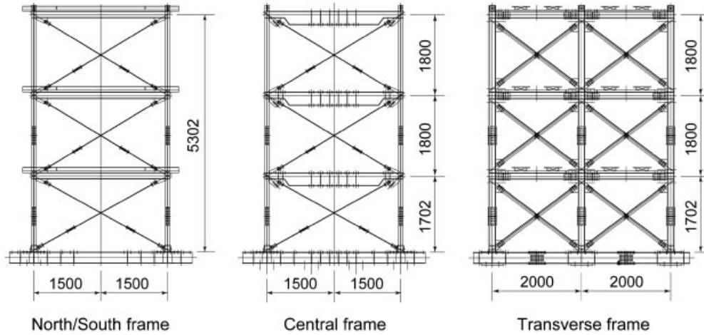
Figure 3. Elevation of test structure.
