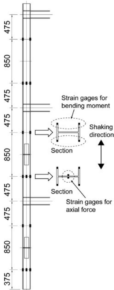
Figure 7. Locations of strain gauges attached to columns.
