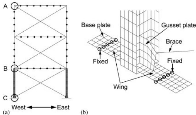
Figure 8. Finite element analytical model: (a) overall frame; and (b) details around base plates.
