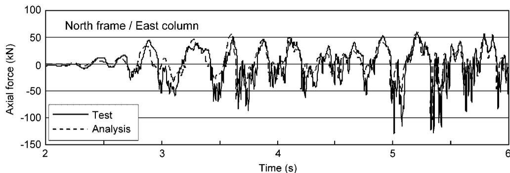
Figure 22. Time histories of axial force variations of column at first storey of BP9-2 model. Maximum input acceleration =  $5.84 \text{ m/s}^2$ .
