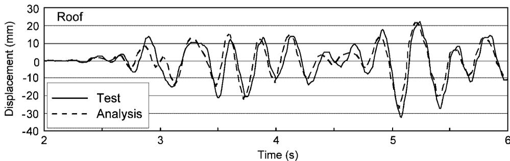
Figure 11. Time histories of roof displacement responses of BP9-2 model. Maximum input acceleration =  $5.84 \text{ m/s}^2$ .
