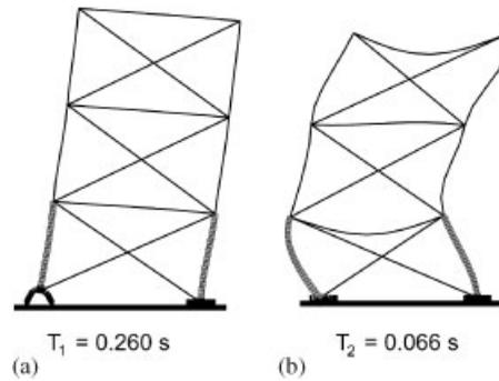
Figure 10. Translational vibration mode shapes in bending: (a) first bending mode; and (b) second bending mode.
