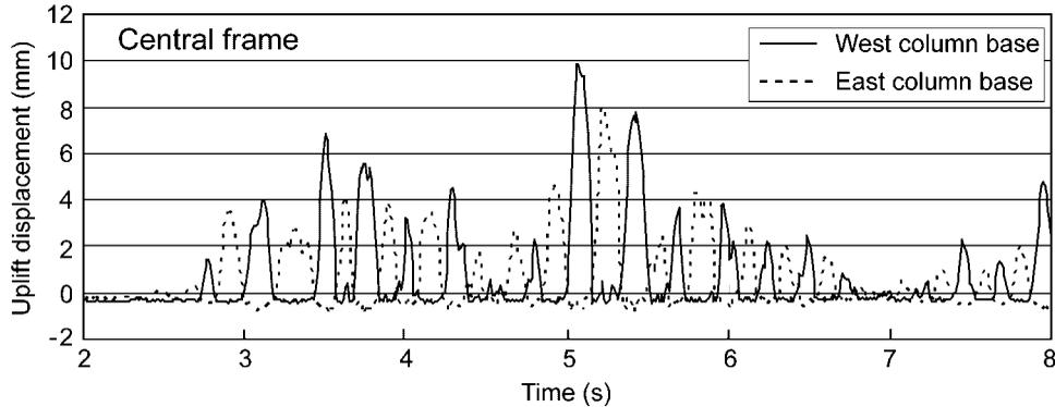
Figure 18. Time histories of uplift displacement responses of BP9-2 model. Maximum input acceleration =  $5.84 \text{ m/s}^2$ .
