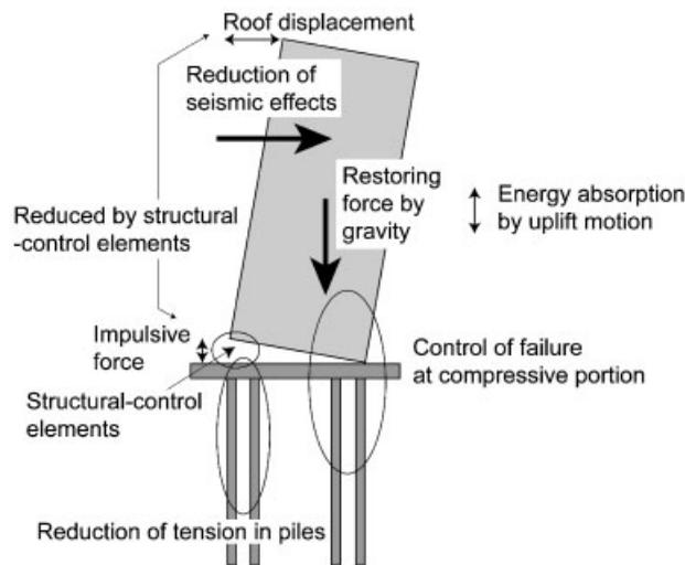
Figure 1. Structural rocking systems.
