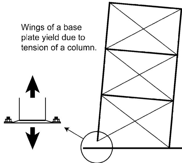
Figure 2. Structural rocking systems with yielding base plates.
