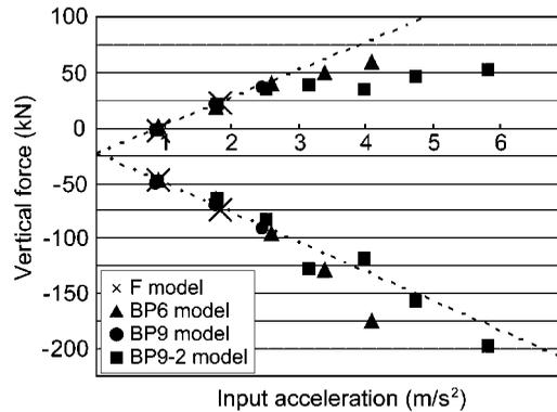
Figure 19. Maximum vertical forces versus maximum input accelerations.
