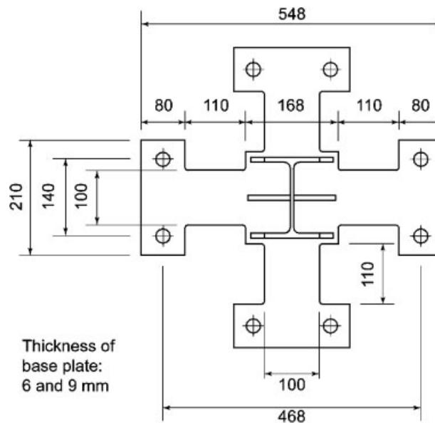
Figure 5. Plan of yielding base plate.
