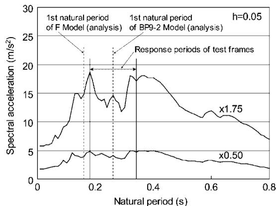
Figure 9. Acceleration response spectra of measured table accelerations.
