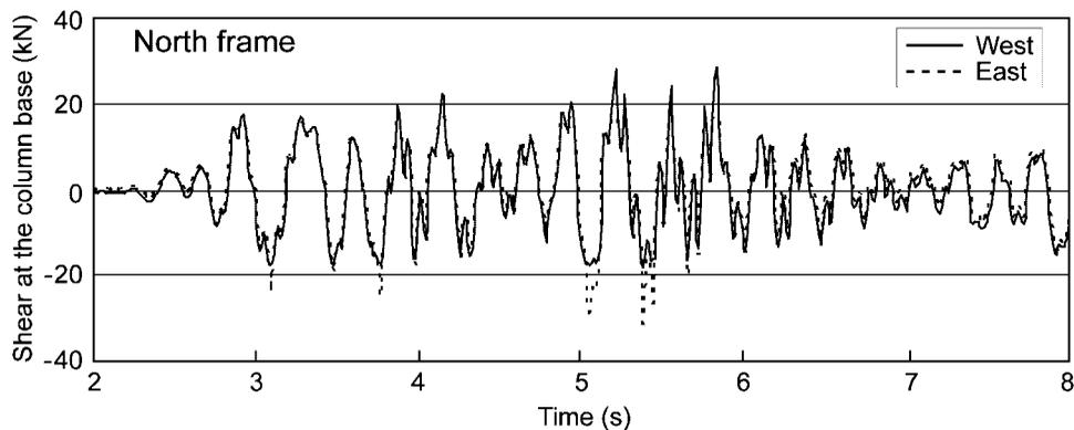
Figure 15. Time histories of shear forces at column bases of BP9-2 model. Maximum input acceleration = 5.84 m/s<sup>2</sup>.
