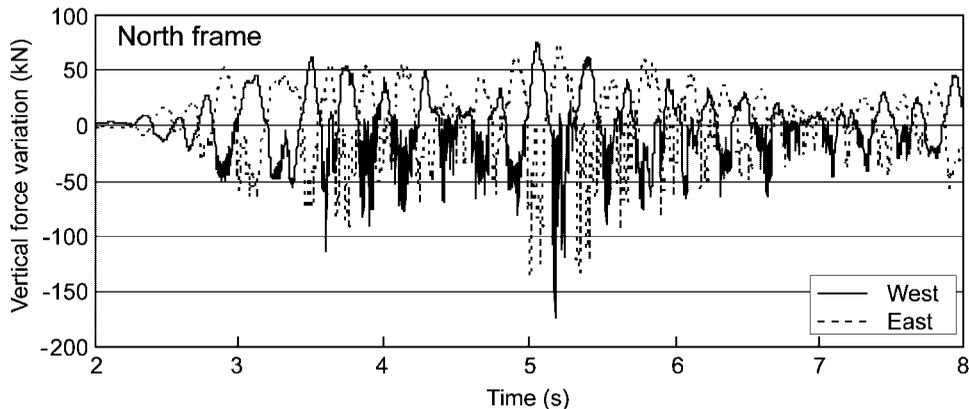
Figure 17. Time histories of vertical force variations at column bases of BP9-2 model. Maximum input acceleration =  $5.84 \text{ m/s}^2$ .
