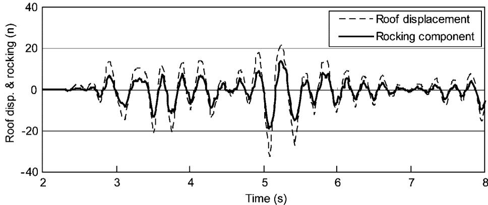
Figure 13. Time histories of roof displacement and rocking component of BP9-2 model. Maximum input acceleration =  $5.84 \text{ m/s}^2$ .
