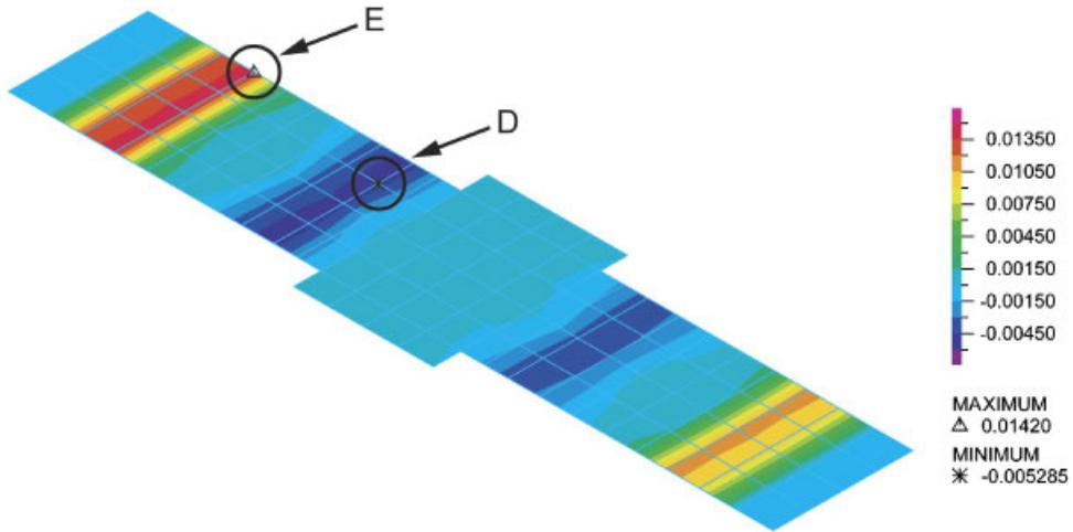
Plate 1. Strain distribution in shaking direction on bottom surface of base plate at west column base of BP9-2 model ( $t = 5.05$  s).
