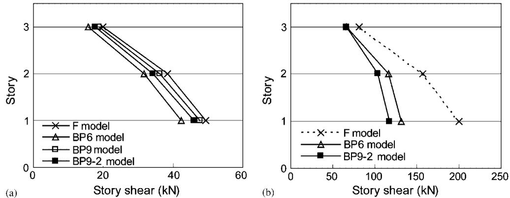
Figure 14. Maximum storey shears of test frames: maximum input acceleration = (a) 0.9 m/s<sup>2</sup>; and (b) 3.5 m/s<sup>2</sup>.
