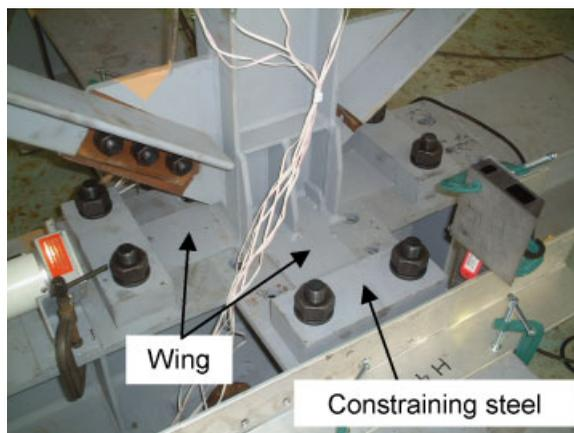
Figure 6. Close-up of yielding base plate.
