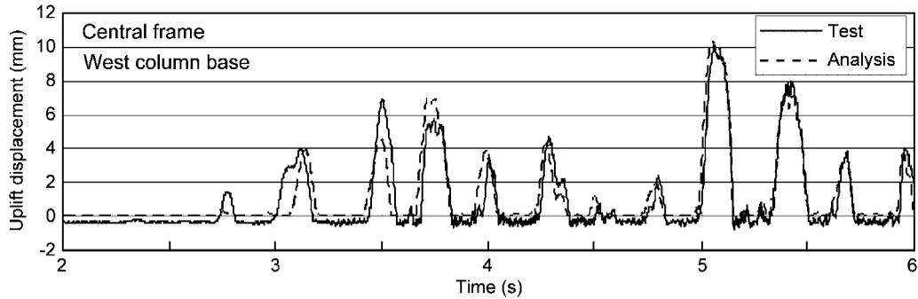
Figure 20. Time histories of uplift displacement responses at column base of BP9-2 model. Maximum input acceleration =  $5.84 \text{ m/s}^2$ .
