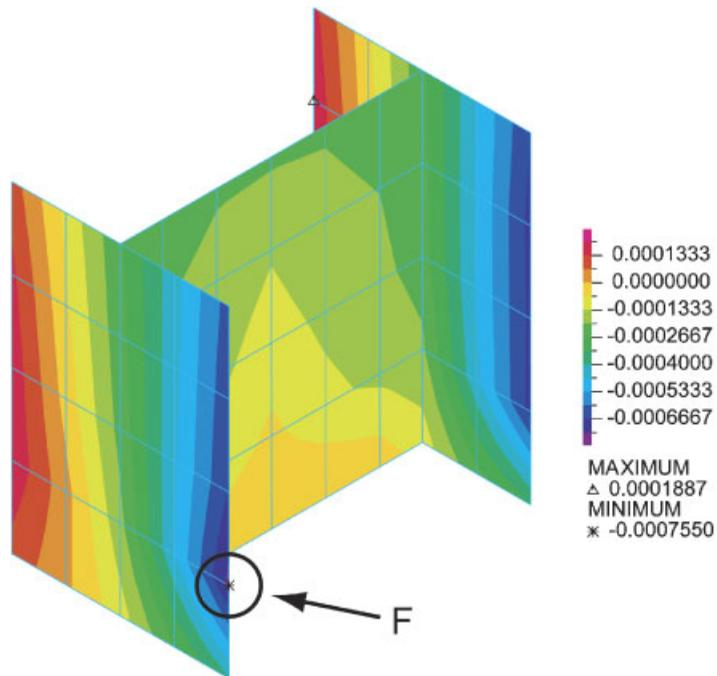
Plate 2. Strain distribution in longitudinal direction on surface at bottom of west column of BP9-2 model ( $t = 5.17$  s).
