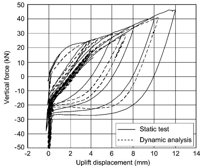
Figure 21. Vertical force versus uplift displacement at west column base of BP9-2 model. Maximum input acceleration =  $5.84 \text{ m/s}^2$ .
