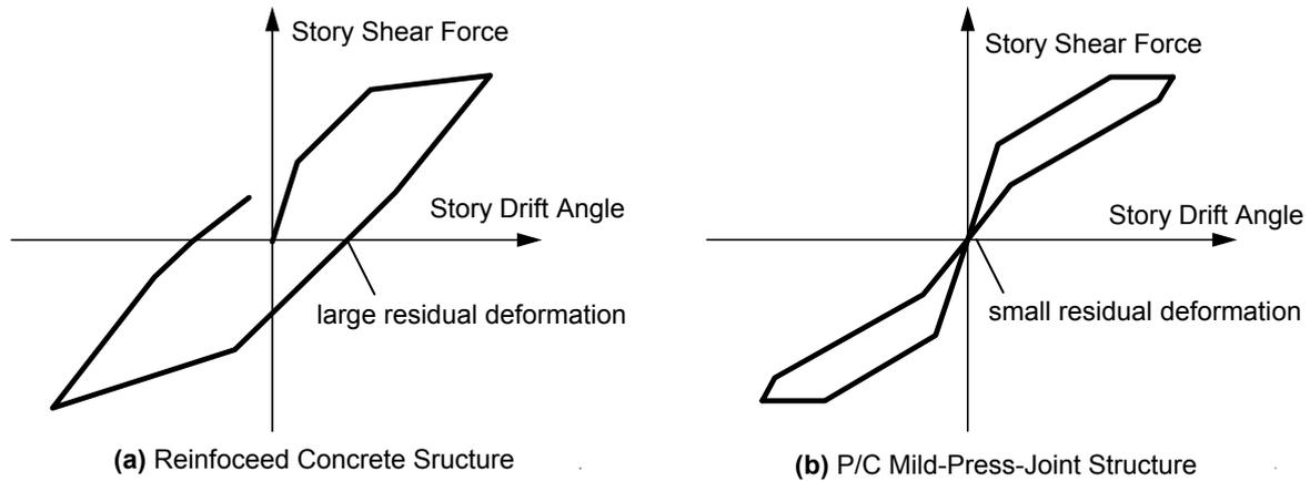
Fig. 1. Compare Reinforced Concrete Structure with P/C Mild-Press-Joint Structure
