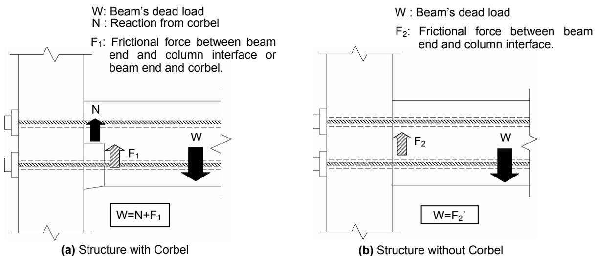
Fig. 3. Difference between with Corbel and without Corbel
