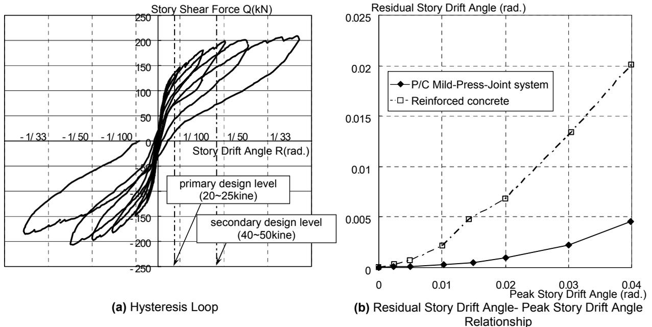
Fig. 6. Deformation Property of P/C Mild-Press-Joint
