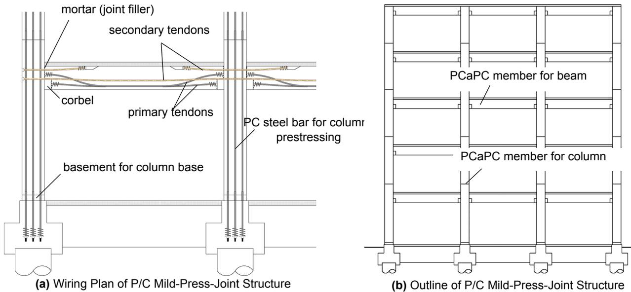
Fig. 2. Example of P/C Mild-Press-Joint Structure
