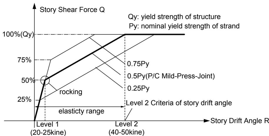
Fig. 9. Conceptual Skeleton Curve of the Frame for Various Levels of Prestress Forces
