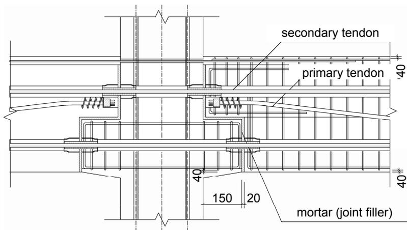
Fig. 8. Detail of Beam-Column Connection
