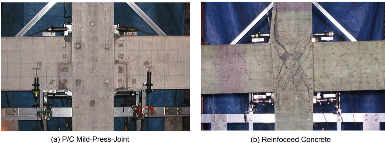
Fig. 7. Ultimate Stage (story drift angle  $R=1/25$  rad.)
