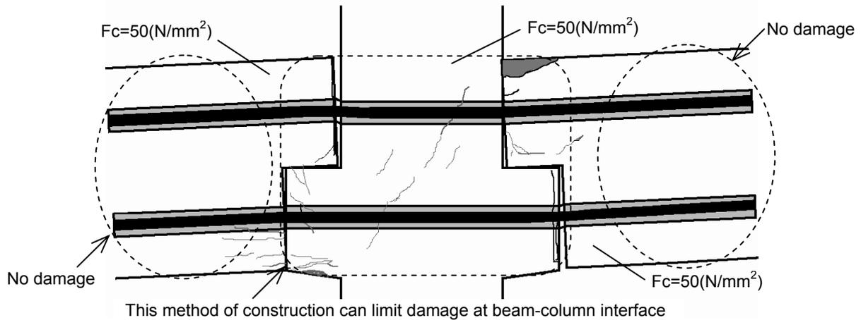
Fig. 4. Ultimate State (P/C Mild-Press-Joint)
