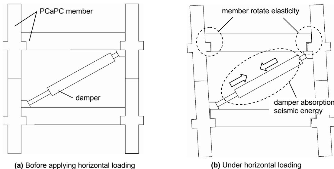
Fig. 5. Example of Energy Absorption in P/C Mild-Press-Joint Structure
