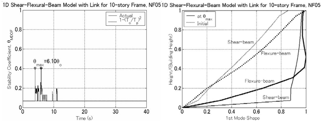
(a)  $P$ - $\Delta$  stability coefficient (b) Instantaneous 1<sup>st</sup>-mode shape
