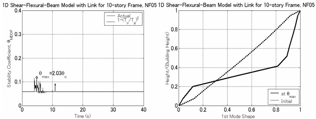
(a)  $P$ - $\Delta$  stability coefficient      (b) Instantaneous 1<sup>st</sup>-mode shape
