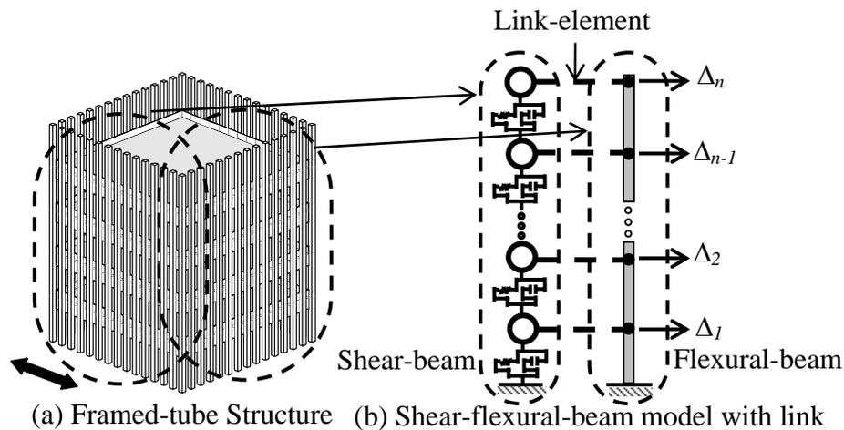
Figure 2: Configuration of 1D coupled shear-flexural-beam model with link.
