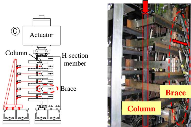
(a) Elevation of specimen and test device (b) Picture of specimen and test device
