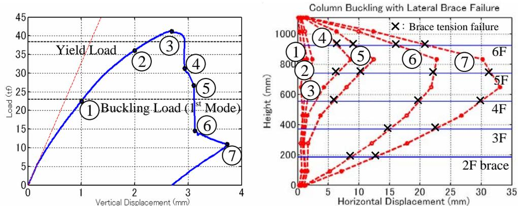
(a) Load - vertical displacement (b) Mode shape of horizontal displacement
