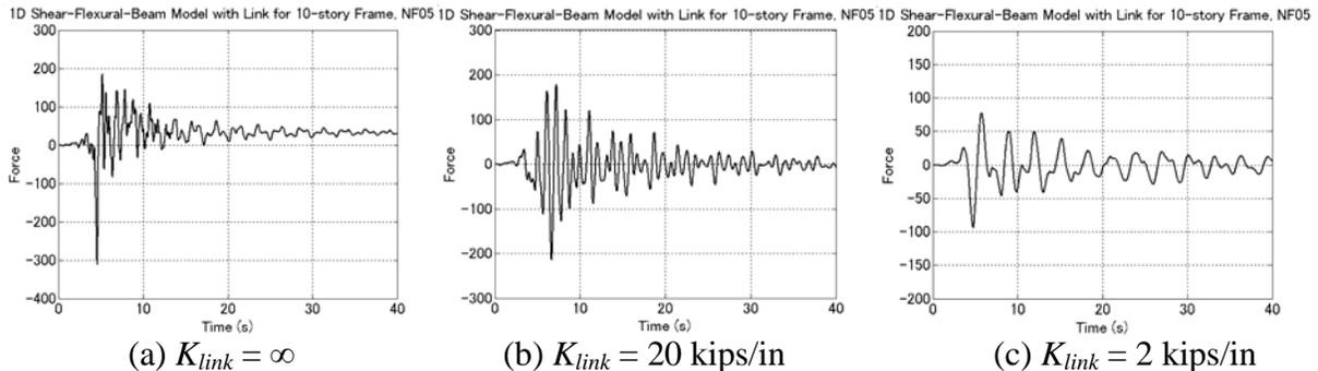
Figure 8: Link-element force histories for 1D MDOF coupled model with various  $K_{link}$ , NF05.
