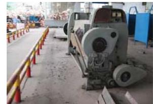
Figure 18. Sliding of un-anchored equipment
