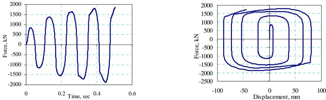
**Fig.6:** Force limit state simulation: force in the damper and unit hysteresis
