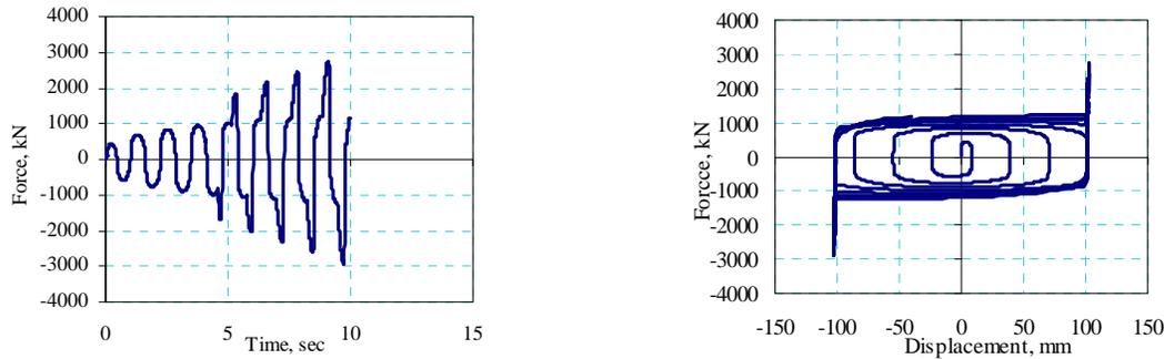
**Fig.7:** Displacement limit state simulation: force in the damper and unit hysteresis
