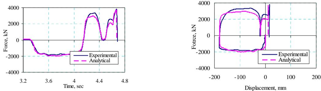
**Fig.9:** Correlation with experimental data: damper force and hysteresis loops
