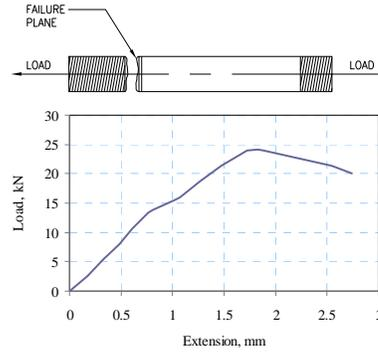
**Fig.5:** Piston undercut and test data
