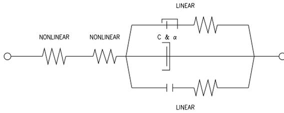
**Fig.4:** Refined model for viscous dampers
