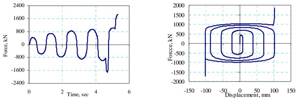
**Fig.8:** Compound limit state simulation: force in the damper and unit hysteresis
