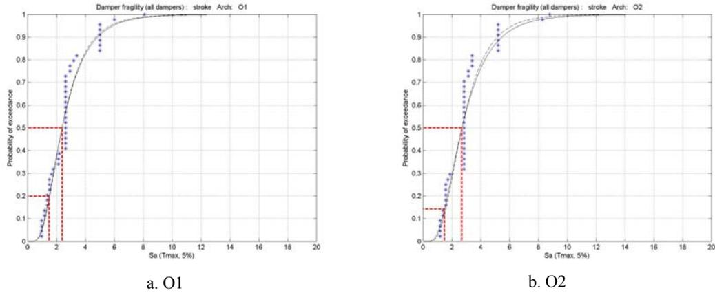
**Figure 14. Damper stroke fragility**
